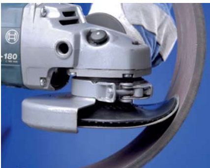
Fiber discs give a particularly soft and flexible abrasive performance in face grinding.
