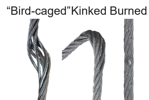
Fig. B: Cable Defects
